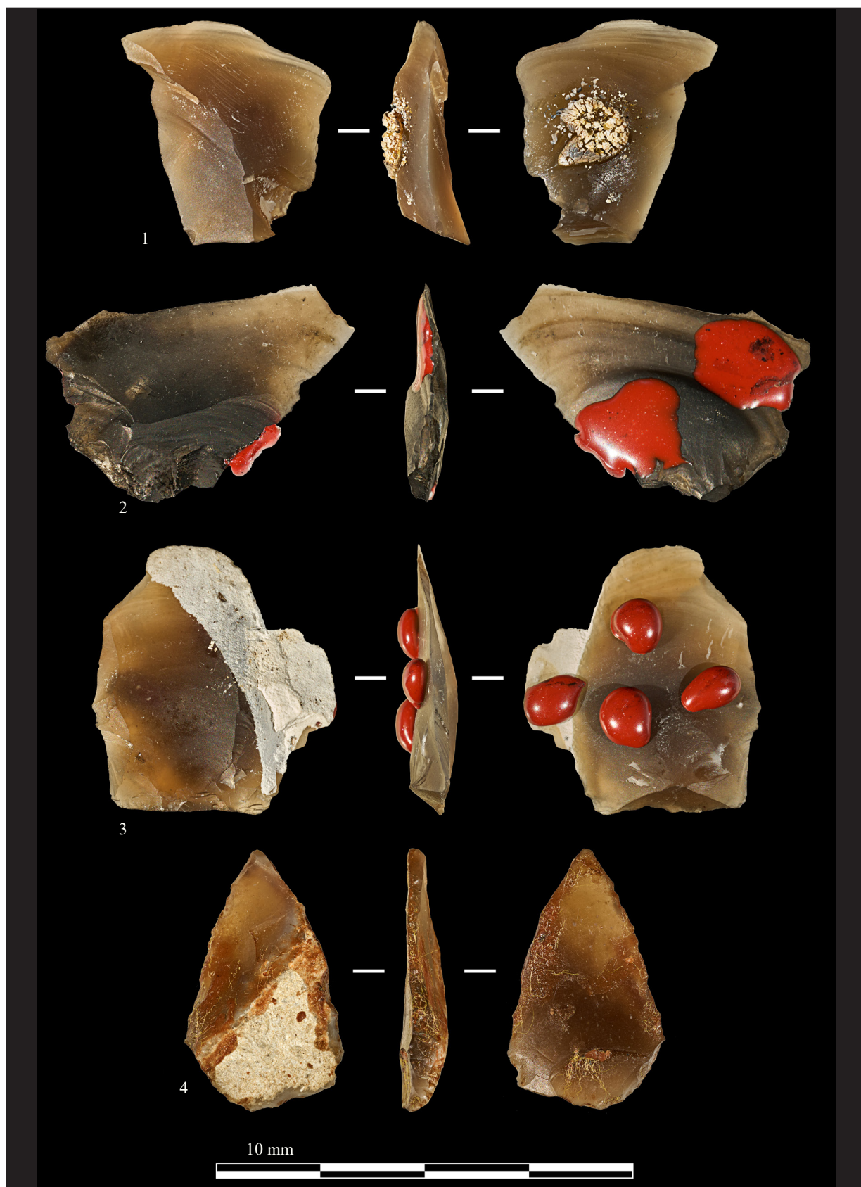
Fig. 7. Experimental data. Examples of experimental objects with hot substances containing pigments applied to their surface. 1–3 — dot applications of polymer glue (1) and sealing wax (2, 3) on flint flakes. The sealing wax does not spread on a cooled surface (3) compared to an object at room temperature (2); 4 — more intensive application of sealing wax on flint flake. To remove the sticky layer, it must be reheated or frozen. After removing the sealing wax, small unevenly coloured spots remain. There are no potlid-like cracks on any experimental object
